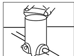
4. Remove temporary cover; measure thickness of floor to be applied and draw a line around the box at this distance from the concrete.
