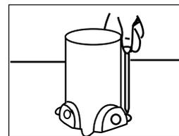
2. Solvent cement conduit into corresponding outlet(s) in box.
