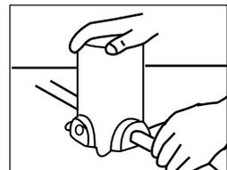
3. Attach temporary cover and seal vacant outlet with solvent-cemented plugs. Pour concrete.
