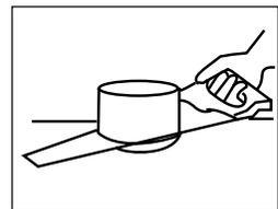
Note: Box may extend above finished concrete. Box is cut to exact height with a handsaw. Leveling ring assures a level top, even if the box is knocked at an angle during the pouring process.
