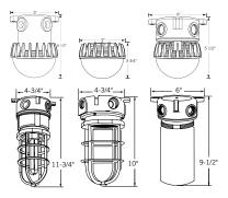
Ceiling Mount Utility Fixtures Box with threaded hubs and integral mounting feet
